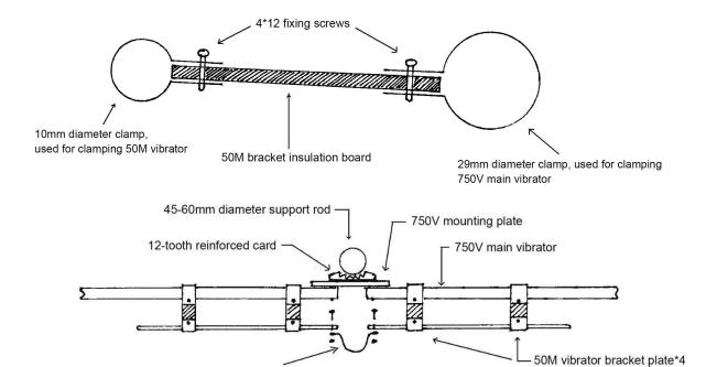
50M vibrator spacing 6-16CM, connecting wire (self-provided) 10-18CM
